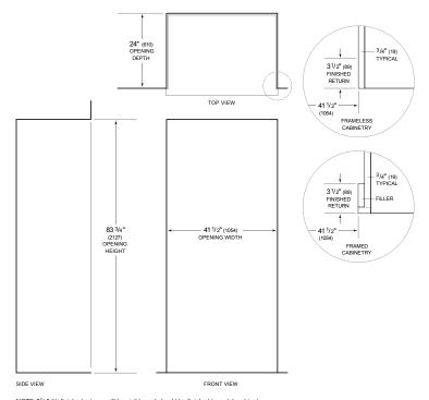
NOTE: 3'/2" (89) finished returns will be visible and should be finished to match cabinetr Shaded line represents profile of unit.
