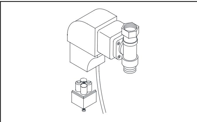
3a. Optional ACA version: Connect supplied inline connector and AC adapter.
