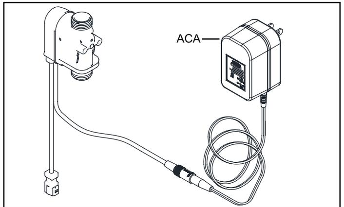
3b. Optional HW6 (Hardwired 6V) version: Connect supplied inline connector and hardwire adapter. When securing the CWB wires to the screw terminals on HW6 unit, the BLACK WITH DASHED MARKINGS should be connected to the Positive (+) terminal, and the SOLID BLACK wire should be connected to the Negative (-) terminal.
