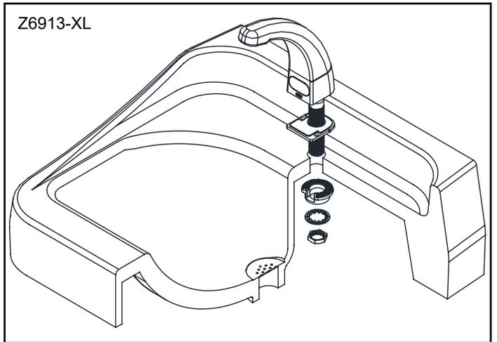
3. Ensure that slot in plastic washer is facing forward.
