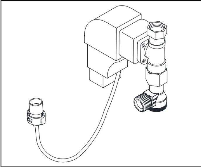
2. For battery-powered version, connect sensor inline connector to electronics module.
