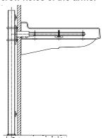
Once the lavatory is set to the proper height and leveled, gradually reverse the lock-down bar screw from the arm until the rubber pads of the lock-down make contact with the fixture, securely locking it into place.
