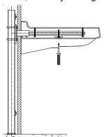
Install lavatory lock-down bar to arm by threading it up through the underside of the arm as shown, keeping the wings of the lock-down in line with the arm.
