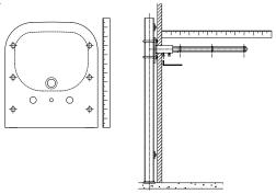
**3** ■ Gently slide lavatory onto the carrier arms to within 1/16" of the finished wall. The access holes on the underside of the lavatory should line up with the lockdown bar & adjustment screw holes of the arms.
