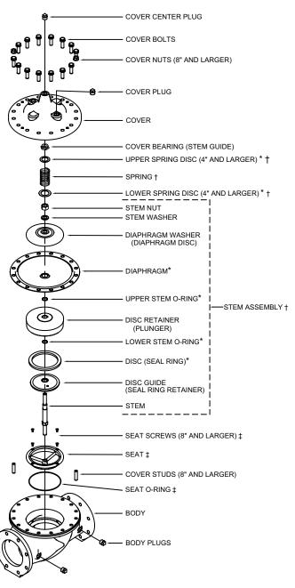
\* RUBBER REPAIR KIT ITEMS † COMPLETE REPAIR KIT ITEMS ‡ SEAT REPAIR KIT
