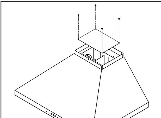
7. From outside hood body, attach top cover plate to top of hood body using (4) M4 x 8 machine screws.
