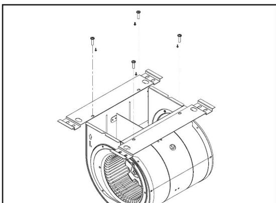
4. Attach rear ducting brackets to motor by (4) previously removed screws from step 1.
