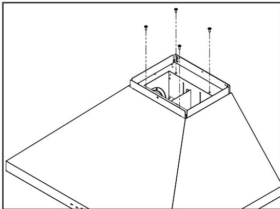
1. Remove (4) screws attaching motor to hood body. Remove the blower and disconnect the blower plug from the hood.
