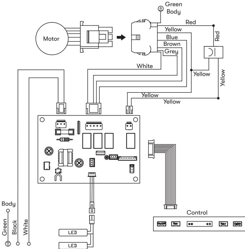
REMARKS: CONDENSER 11+11uF 250VAC FIT AC120V 60Hz
