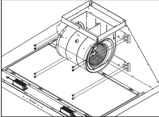
6. Attach motor to back of hood body by (8) 3/16" x 3/8" screws and reconnect the blower plug.
