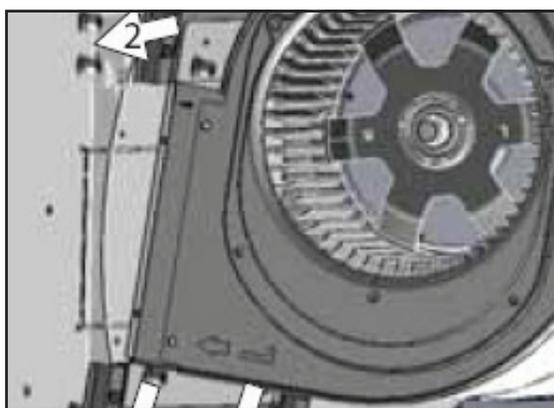
5. Position blower with brackets as shown. Be sure to tuck back of blower bracket into tabs at back of hood.
