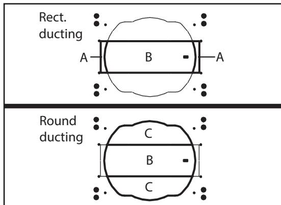
2. Remove knock out plates A & B for rectangular ducting or knock out plates B & C for round ducting with a flat head screwdriver and a rubber mallet.
