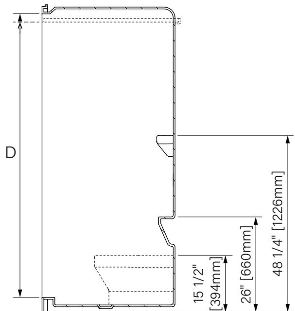
The dotted measurements illustrate the domeless configuration dimensions.
