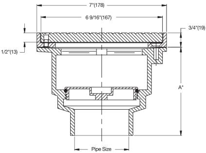
Load Rating \*XHD \* The load classifications are in accordance with the American National Standards ASME A112.21.1M ASME Ratings are as follows:
