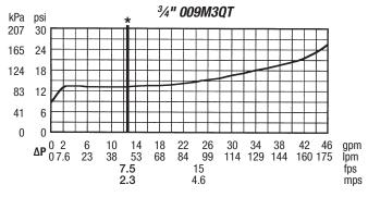
The asterisk (\*) indicates typical maximum system flow rate (7.5 ft/sec, 2.3 m/sec).
