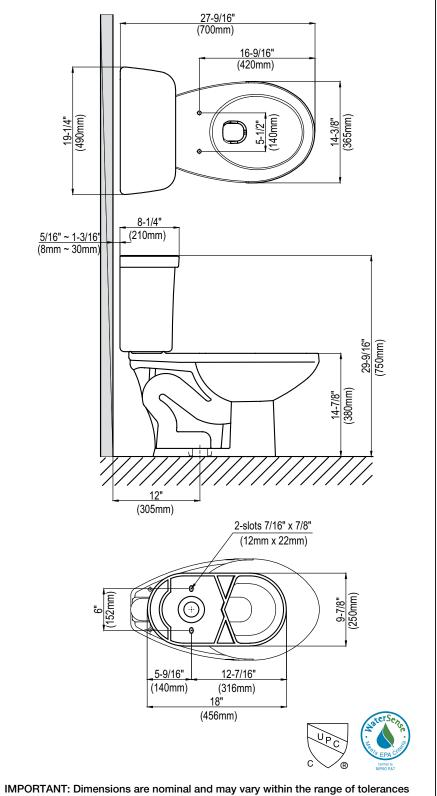
IMPORTANT: Dimensions are nominal and may vary within the range of tolerances established by ASME A112.19.2 / CSA B45.1. These measurements are subject to change without notice.
