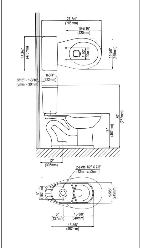
IMPORTANT: Dimensions are nominal and may vary within the range of tolerances established by ASME A112.19.2 / CSA B45.1. These measurements are subject to change without notice.
