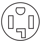
4-wire receptacle (14-30R)
