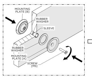
Insert the SLEEVE into the pre-drilled hole then reassemble the ADAPTER using the SCREW provided.
