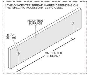
. Ensure any pre-drilled hole is a 1/2" [13mm]. For ACCESSORIES with 2 mounting holes, ensure the holes are level and at the proper on-center spread.
