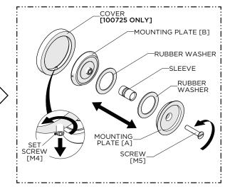
Disassemble the components by unthreading the SCREW on the MOUNTING PLATE [A].
