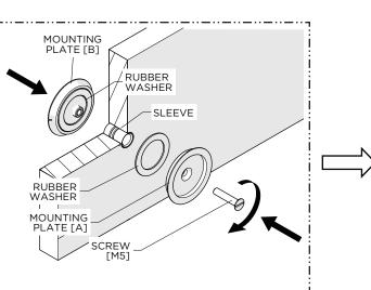
Insert the SLEEVE into the pre-drilled hole then reassemble the ADAPTER using the SCREW provided.
