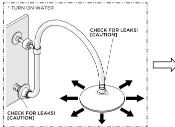
8. Turn on the water and operate the SHOWER HEAD to ensure it pivots and functions properly. Inspect all connections for leaks then turn the water off.
