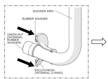
4. Slide the INLET ESCUTCHEON and RUBBER WASHER up the SHOWER ARM to expose the UNION NUT.
