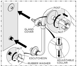
Align the NUT to the NIPPLE and the POST to the WALL BRACKET then thread and securely tighten the NUT onto the NIPPLE making sure the POST fits properly onto the WALL BRACKET.
