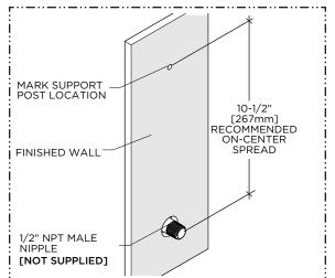
2. Mark the location for the SUPPORT POST from the center of the NIPPLE to the desired on-center spread.
