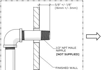
Ensure the front face of the 1/2" NPT MALE NIPPLE (not supplied) is 5/8" [16mm] to +/- 1/8" [3mm] in front of the finished wall.
