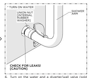
separately) to flush out any debris in the supply line and inspect all connections for leaks then turn the water off.
