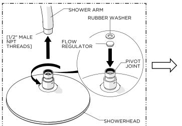
Insert the RUBBER WASHER into the PIVOT JOINT on the SHOWER HEAD then thread and securely tighten the PIVOT JOINT onto the SHOWER ARM.
