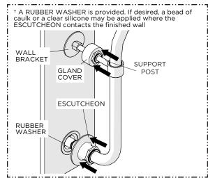
Slide the ESCUTCHEON down the SHOWER ARM until it contacts the finished wall and slide the GLAND COVER down the SUPPORT POST until it contacts the WALL BRACKET.
