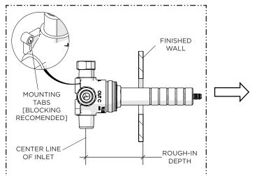
The VALVE rough-in depth is measured from the center of the inlets to the surface of the finished wall and VARIES depending on the TRIM used.
