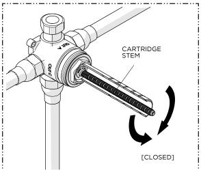
After the supply lines have been fully flushed, turn off the water.
