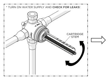
Turn on the water supply and operate the CARTRIDGE STEM to flush out the lines and check for leaks.
