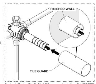
Install the TILE GUARD to protect the DIVERTER VALVE during the completion of the finished wall and to create the exact opening required to ensure access to the CARTRIDGE for future servicing.
