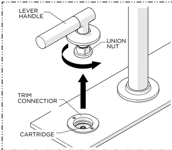
2. Unthread the UNION NUT from the TRIM CONNECTOR to expose the CARTRIDGE.
