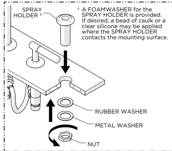
11. Insert the SPRAY HOLDER through the hole on the mounting surface then re-install the WASHERS and securely tighten the NUT.
