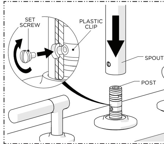
2. When replacing the SPOUT, the SET SCREW must properly align with the hole on the PLASTIC CLIP to securely hold the SPOUT in position.
