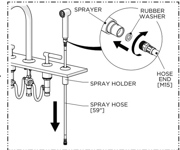
12. Using the RUBBER WASHER provided, thread one end of the SPRAY HOSE into the SPRAY HOLDER then insert the SPRAY HOSE through the SPRAY HOLDER.
