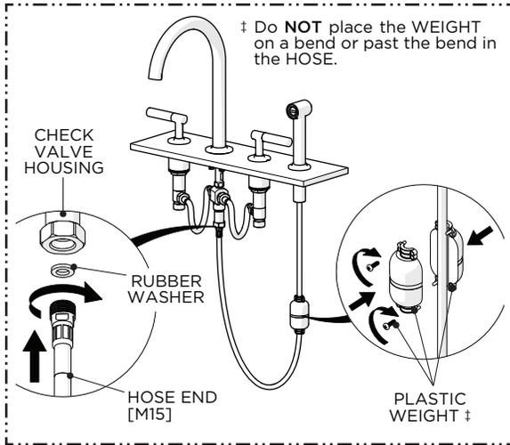
13. Using the RUBBER WASHER provided, thread the SPRAY HOSE into the CHECK VALVE HOUSING then attach the WEIGHT to a **straight** section of the HOSE that is opposite the HOUSING/TEE and verify the SPRAYER sits properly in the HOLDER.
