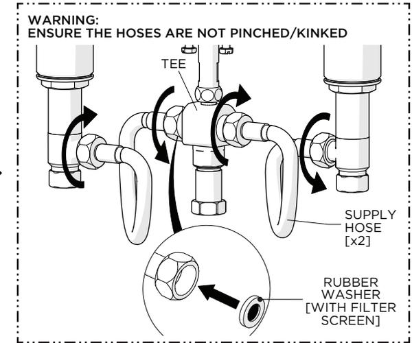
9. Connect the SIDEBODIES to the TEE using the SUPPLY HOSES and WASHERS provided. Securely tighten the HOSES and ensure they are not pinched/kinked.
