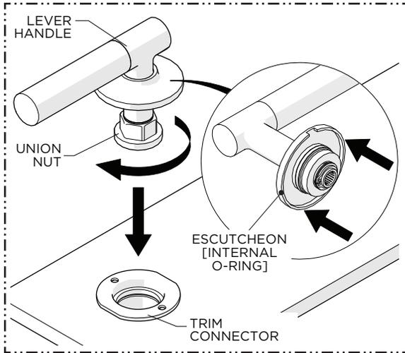
7. **CAREFULLY** slide the ESCUTCHEON up the LEVER HANDLE to expose the UNION NUT then thread the NUT into the TRIM CONNECTOR until it stops.
