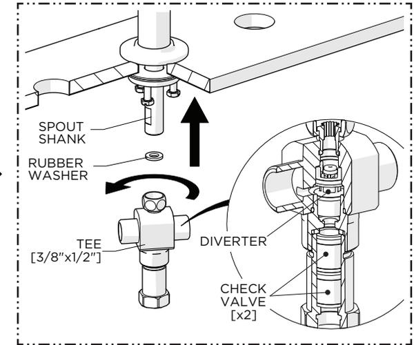
3. Using the RUBBER WASHER provided, thread and securely tighten the TEE onto the SPOUT SHANK.
