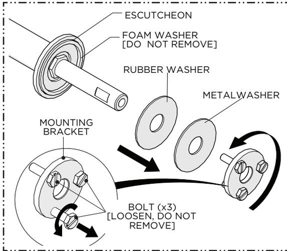
1. Unthread and remove the MOUNTING BRACKET, and WASHERS from the SPOUT SHANK then loosen the BOLTS on the BRACKET.
