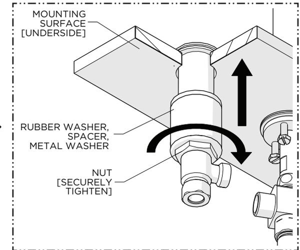
6. Ensure the SIDEBODY is positioned so the SUPPLY HOSE can be easily connected to the TEE then thread and securely tighten the NUT against the underside of the mounting surface.
