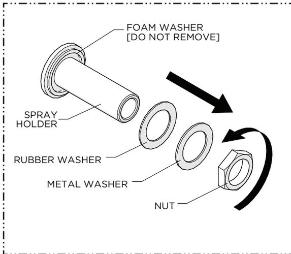
10. Remove the NUT, METAL WASHER, and RUBBER WASHER from the SPRAY HOLDER.
