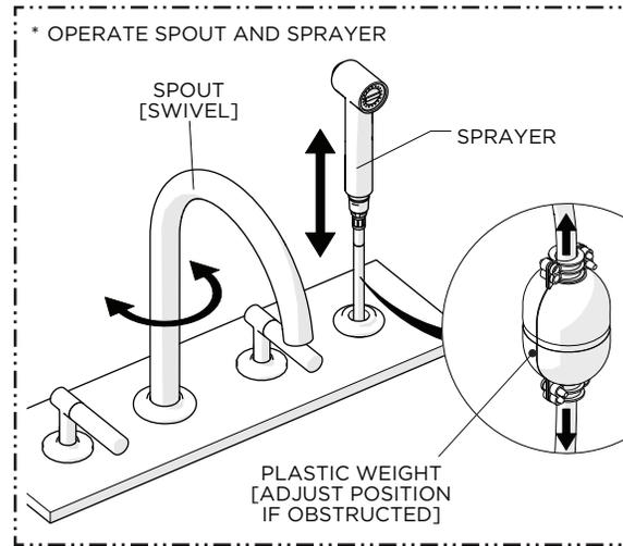
17. Pull out the SPRAYER and rotate the SPOUT to ensure they function properly and the WEIGHT can move freely beneath the cabinet.
