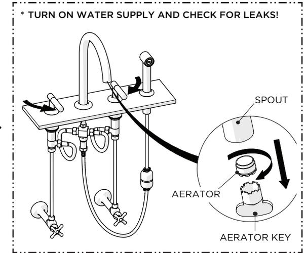
15. Unthread and remove the AERATOR then turn on the water supply and open the FAUCET to flush out any debris in the supply lines prior to operating the SPRAYER. Inspect all connections for leaks.
