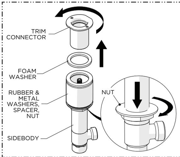
4. Unthread and remove the TRIM CONNECTOR and FOAM WASHER from the SIDEBODY then fully thread the NUT down the SIDEBODY.
