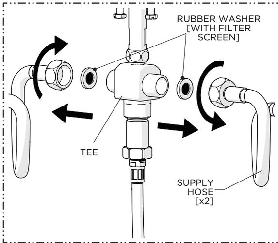
16. Turn off the FAUCET and unthread both the SUPPLY HOSES from the TEE to remove and clean the WASHER WITH FILTER SCREENS then re-install the WASHERS and HOSES.
