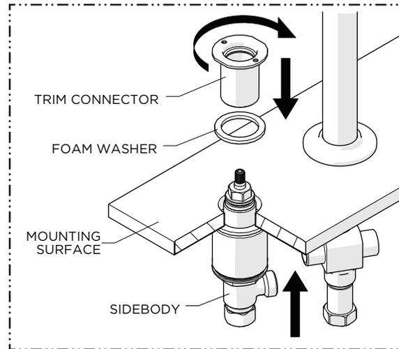
5. Insert the SIDEBODY into the hole on the mounting surface from below then, using the FOAM WASHER provided, thread the TRIM CONNECTOR back onto the SIDEBODY until it stops.
