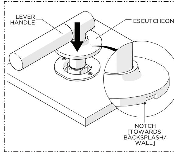
8. **CAREFULLY** slide the ESCUTCHEON down the LEVER HANDLE to conceal the TRIM CONNECTOR.
