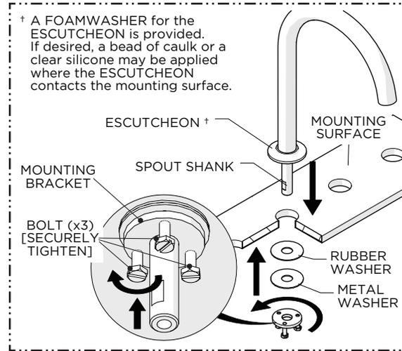
2. Insert the SPOUT SHANK through the hole on the mounting surface then re-install the WASHERS and MOUNTING BRACKET.
