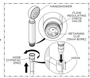
Thread the conical end of the HOSE to the HANDSHOWER then rest the HANDSHOWER on the HOOK.
