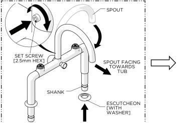
Align the SPOUT properly and securely tighten the SET SCREW at the base of the SPOUT then slide the ESCUTCHEONS onto the SHANKS.
