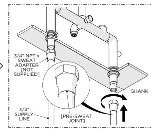
3. Pre-sweat 3/4" female NPT x sweat adapters to 3/4" supply lines and let cool. Apply a thin coat of pipe thread sealant to the male threads on the SHANKS then thread and securely tighten the ADAPTERS onto the SHANKS.
