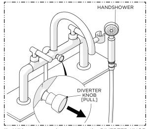
11. With water running, operate the DIVERTER KNOB to ensure it and the HANDSHOWER function properly then turn off the water.
