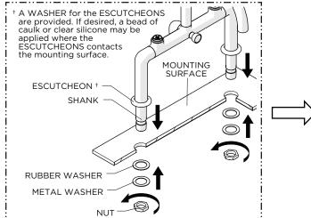
Insert the SHANKS into the holes on the mounting surface then attach the RUBBER and METAL WASHERS and NUTS onto the SHANKS. Securely tighten the NUTS against the underside of the mounting surface.
