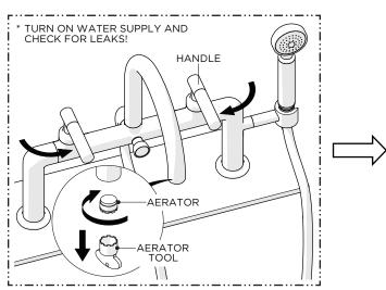
Remove the AERATOR using the TOOL provided then turn on the water supply and operate the HANDLES to flush out the supply lines and check all connections for leaks.
