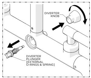
While holding the DIVERTER PLUNGER, unthread the KNOB from the PLUNGER then remove both parts.
