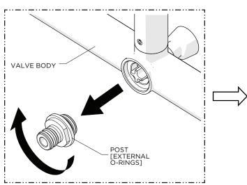
Unthread and remove the POST from the VALVE BODY.
