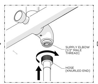
8. Thread the KNURLED END of the HOSE to the SUPPLY ELBOW on the VALVE BODY.
