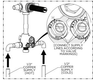
3. Run 1/2" copper supply lines to the proper height and depth of the VALVE INLETS making sure they are piped according to the VALVE markings and all piping and fittings are properly secured.
