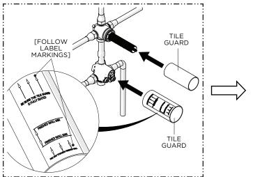
Following the label markings, firmly push both TILE GUARDS onto the VALVE making sure they are FULLY seated.
