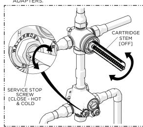
After the supply lines have been fully flushed, turn off the water and close both SERVICE STOPS.
