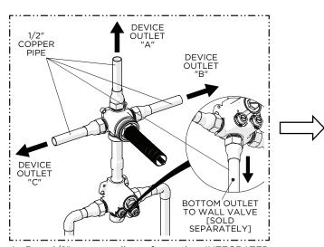
Run 1/2" copper lines from the INTEGRATED DIVERTER VALVE outlets, and bottom outlet if used, to the desired end fittings (sold separately) making sure to secure all piping and fittings.
