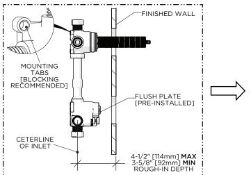
The rough-in depth is measured from the centerline of the inlets to the surface of the finished wall and must be between 4-1/2" [114mm] MAXIMUM and 3-5/8" [92mm] MINIMUM.
