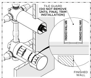
8. Do **NOT** remove the TILE GUARDS until final TRIM installation to ensure the finished wall is within the **MAXIMUM** and **MINIMUM** markings on the TILE GUARD.
