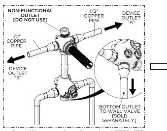
4. Run 1/2" copper lines from the INTEGRATED DIVERTER VALVE outlets, and bottom outlet if used, to the desired end fittings (sold separately) making sure to secure all piping and fittings.
