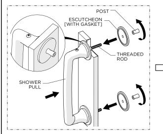
3. While holding the PULL against the mounting surface, slide the ESCUTCHEONS onto the THREADED RODS then thread and securely tighten the RETAINING POSTS onto the RODS.
