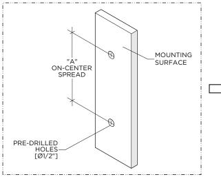
1. Drill two 1/2" diameter holes on the mounting surface at the required on-center spread (DIM A).
