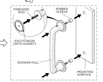
Insert the RUBBER SLEEVES into the pre-drilled holes then slide the ESCUTCHEONS over the THREADED RODS on the PULL and insert the RODS through the RUBBER SLEEVES.
