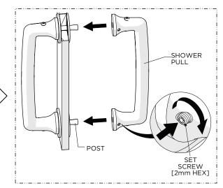
4. Slide the 2nd PULL onto the RETAINING POSTS until it contacts the ESCUTCHEONS then thread and securely tighten the SET SCREWS.
