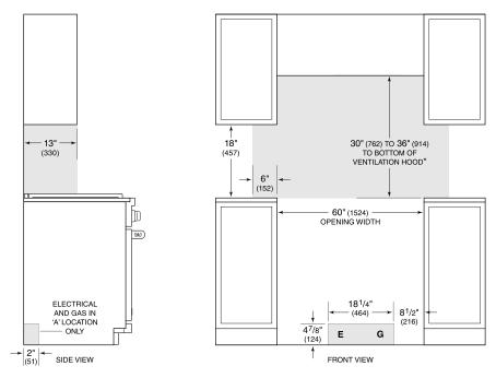
\*Without ventilation hood, 36" (914) minimum clearance countertop to combustible materials, 44" (1118) for charbroiler. NOTE: Shaded area above countertop indicates minimum clearance to combustible surfaces,
