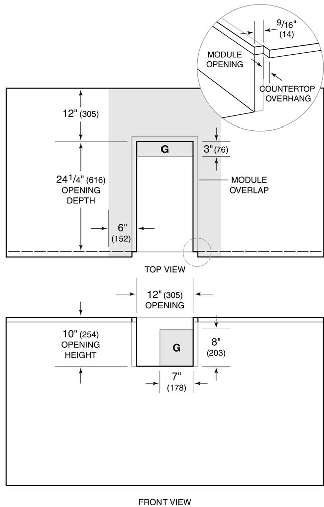
NOTE: Shaded area above countertop indicates minimum clearance to combustible surfaces, combustible materials cannot be located within this area. An insulating liner is not required.
