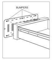
10 Install the mounting panel using six  $^{3}/_{8}$ " screws.
