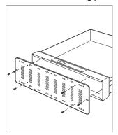
Align the pilot holes on the custom panel with the holes on the mounting panel and attach using <sup>1</sup>/<sub>2</sub>" screws.
