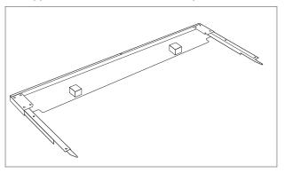
6 Place the center support bracket on a protected work surface, then place the back panel on the center support and install one #8 x 1/2" screw in the back panel bottom hole.
