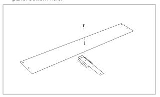
7 Remove the paper backing from the black tape on the center support flanges, then align the center support hole with the center hole on the front panel.
