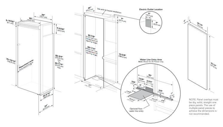
\*Custom panel models fit flush in 25" (63.5 cm) deep cabinet openings. They can be installed in standard 24" (61.0 cm) deep openings. The door faces and top grille will protrude 3/4" (1.9 cm) into the room.
