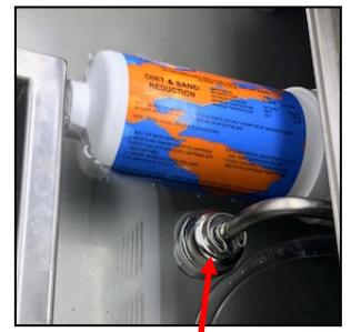
Fig. 2 Float switch/sensor; right side of reservoir; shuts off water once filled to proper level
