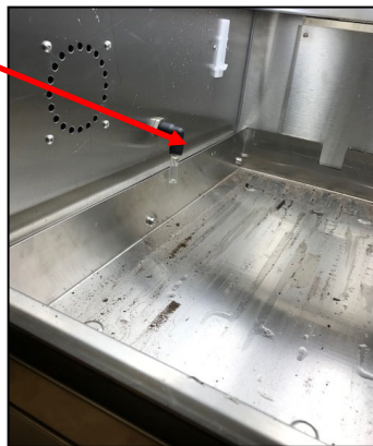
Fig. 5 Zone irrigation nozzle
