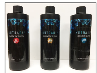
PH kit: PH#4 and PH#7 bottles to calibrate the pH probe.
