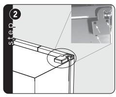
Remove plastic caps from the top hinges by removing (3) 1/4" hex head screws. Save these screws to replace plastic caps.
