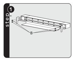
Attach spacers, included in the kit, to the grille assembly with four screws. DO NOT install spacers if installing the side trim.
