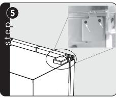
Place plastic caps back on top of hinges and located exisiting holes. Insert screws making sure the grille is centered.
