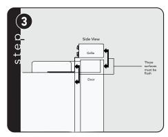
Align and position grille on top of unit so that the face of the grille and the face of the door are flush.
