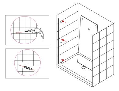
**3.2** - Install the wall profile into place.
