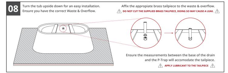
Once the tailpiece is been installed on the waste & overlow, position the Tub and tailpiece in-line with the drain. Carefully lower the tub with the installed brass tailpiece as vertical as possible into the red collar in drain assembly.
