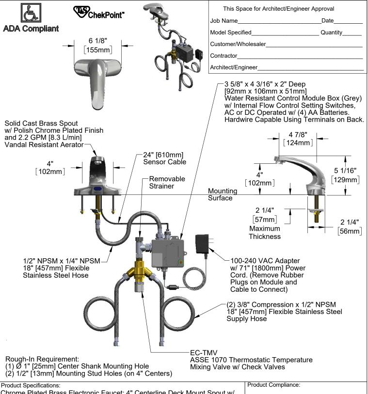
Chrome Plated Brass Electronic Faucet: 4" Centerline Deck Mount Spout w/ 2.2 GPM VR Aerator, AC/DC Control Module w/ Internal Flow Control Setting Switches, Thermostatic Temperature Control Mixing Valve w/ Check Valves, 18" Hot & Cold Flexible Supply Hoses
