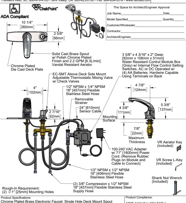
Chrome Plated Brass Electronic Faucet: Single Hole Deck Mount Spout w/ 2.2 GPM VR Aerator, 8" Centers Deck Plate, Above Deck Side Mount Adjustable Thermostatic Mixing Valve w/ Check Valves, AC/DC Control Module with Internal Flow Control Setting Switches, 18" Hot & Cold Supply Stop Flexible Connector Hoses
