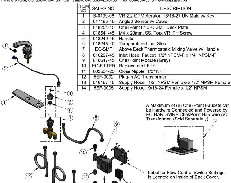
Label for Flow Control Switch Settings is Located on Inside of Back Cover.
