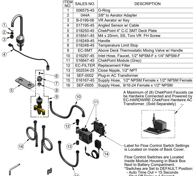
A Maximum of (8) ChekPoint Faucets can be Hardwire Connected and Powered by EC-HARDWIRE ChekPoint Hardwire AČ Transformer. (Sold Separately)
