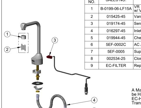
B-0199-06-LF15A VR 1.5 GPM Laminar Flow Device (Anti-Microbial) w/ VR Key
