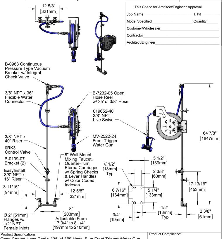
Open Coated Hose Reel w/ 35' of 3/8" Hose, Blue Front Trigger Water Gun w/ Swivel, Vacuum Breaker, 3/8" NPT Flexible Water Connector, 8" Wall Mount Faucet, & Control Valve
