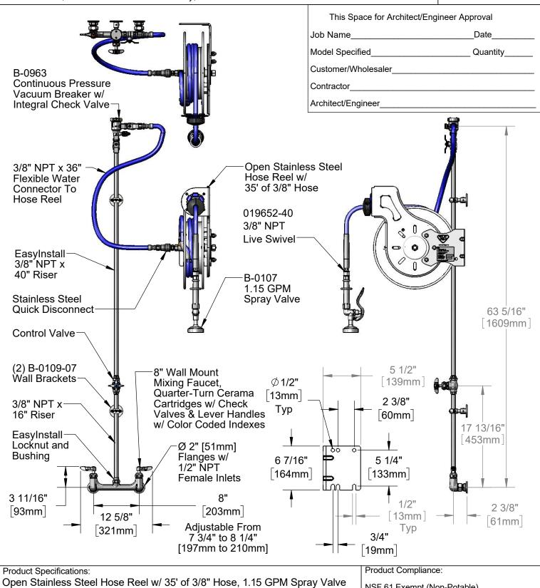
Open Stainless Steel Hose Reel w/ 35' of 3/8" Hose, 1.15 GPM Spray Valve w/ Swivel, Vacuum Breaker, 3/8" NPT Flexible Water Connector, 8" Wall Mount Mixing Faucet w/ Quarter-Turn Cerama Cartridges & Control Valve
