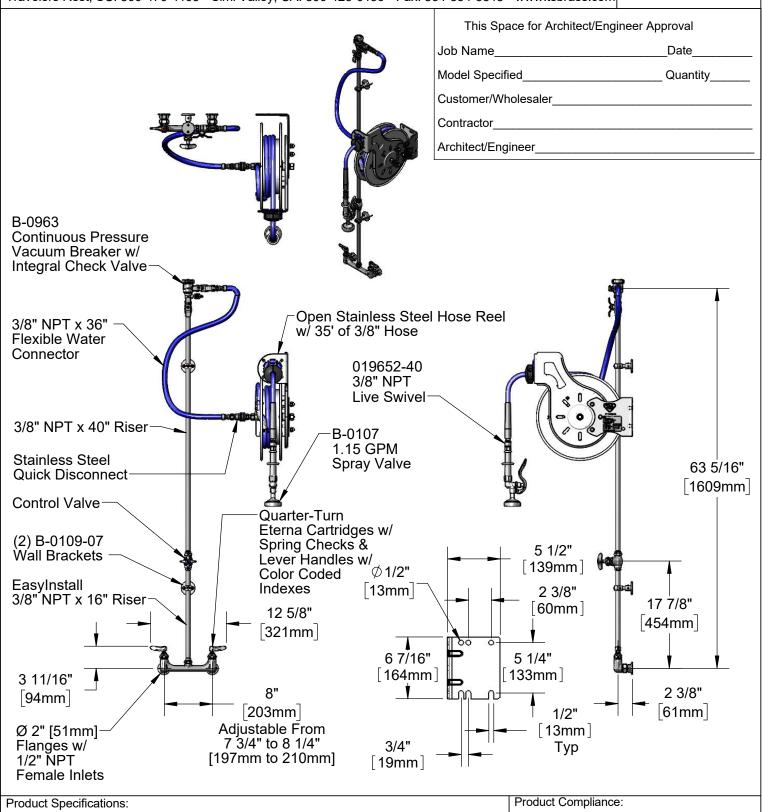
Open Stainless Steel Hose Reel w/ 35' of 3/8" Hose, 1.15 GPM Spray Valve w/ Swivel, Vacuum Breaker, 3/8" NPT Flexible Water Connector, 8" Wall Mount Mixing Faucet & Control Valve
