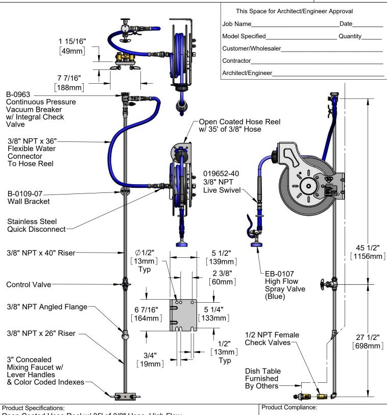
Open Coated Hose Reel w/ 35' of 3/8" Hose, High Flow Spray Valve (Blue) w/ Swivel, Vacuum Breaker, 3/8" NPT Flexible Water Connector, 3" Concealed Mixing Faucet & Control Valve
