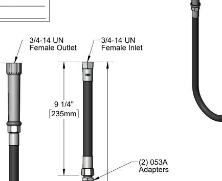
(2) 010476-45 Washers (Included) B-0970-FE Continuous Pressure Atmospheric Vacuum Breaker 44" [1117mm]
