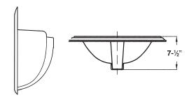
Dimensions shown for location of supplies, waste and mounting clips are suggested. Installation instructions supplied with lavatory. Mounting clips included.
