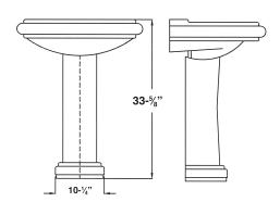
Dimensions shown for location of supplies, waste and mounting clips are suggested. Installation instructions supplied with lavatory. Mounting clips included.
