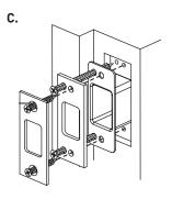
Match screw holes on strike with vertical center lines on jamb. Mark outline of strike and chisel 1/4" (6.4 mm) deep for flush fit of dust box, wood frame reinforcer, and strike. Place dust box and wood frame reinforcer into mortise area ad tighten to the frame using 3" wood screws. Insert the strike and tighten to the frame with #8 screws.
