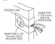
Measure center line of lock; height as desired from finished floor. Select 2-3/4" or optional 2-3/8" backset, fold and apply template to interior side of door and mark center of door as indicated on template. Mark center hole on door face through guide on template.
