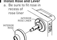
b. Depress lever catch with tool provided. Push interior lever in completely until catch engages in lever. Confirm lever is INTERIOR secured.
