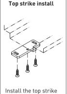
to the frame with 3 screws as shown.
