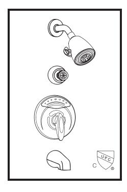
**SYMMONS PRODUCTS MEET** ASME A112.18.1/ CSA B125.1 AND ALL KNOWN FLOW RATE REQUIREMENTS. Shower Heads and Hand Showers 2.5 GPM (9.5 L/min)
