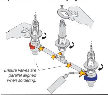
Step 3 Mount valve assembly to deck
