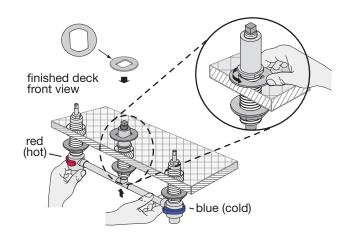
Step 4 Attach valve assembly to deck
