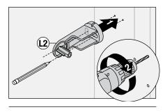
**Option:** Place mounting plate (L2) in position, mark and drill 3/16" holes into wall. Install anchors.
