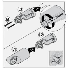
**Note:** Mounting plate (L2) center tabs must be horizontal for installation.
