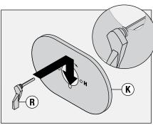
Install shower escutcheon (K) to shower valve. Secure with two screws (J).
