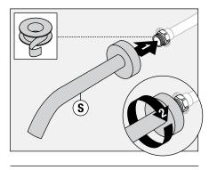
6) Install wall elbow (B) and flange (C) to recessed pipe fitting. Turn elbow clockwise to tighten.
