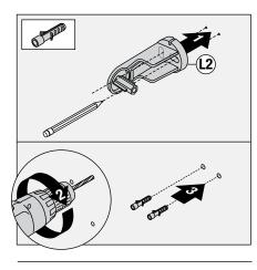
9) Install mounting plate (L2). Secure with two screws (M). Replace cradle mount cover (L1).
