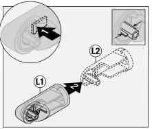
**Note:** Mounting plate (L2) center tabs must be horizontal for removal.
