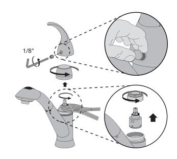
Replacing cartridge and handle
