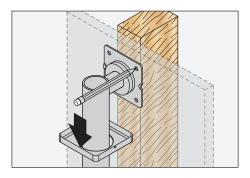
Place bar at desired position. Slide covers over bar to reveal flanges. Mark drill hole locations with pencil at each end on inner side of flanges.
