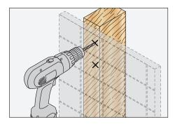
1) Use drill with 1/4" carbide tip drill bit to drill holes into ceramic tile at the marked positions to prevent damage to the tiles.
