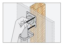
Align mounting holes on bar flanges with drill holes. Insert wood screws into pilot holes for wall and wall studs. Hand tighten wood screws.
