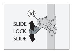
Adjust screw cap 1d for ease of movement of slide mechanism.
