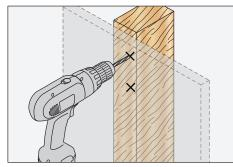
Remove bar from wall. Use drill with 7/64" drill bit to drill holes into wall and wall studs at the marked positions.
