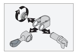
1) Disassemble slide mechanism as shown above.
