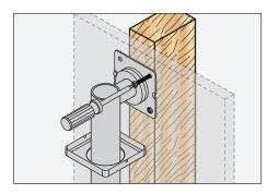
4) Tighten all wood screws using a phillips head screwdriver, securing bar to wall.
