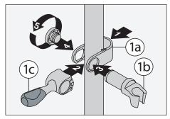
Install slide mechanism to bar.
