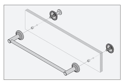
Note: Apply a bead of silicone around the perimeter of trim installed flush to finished wall.
