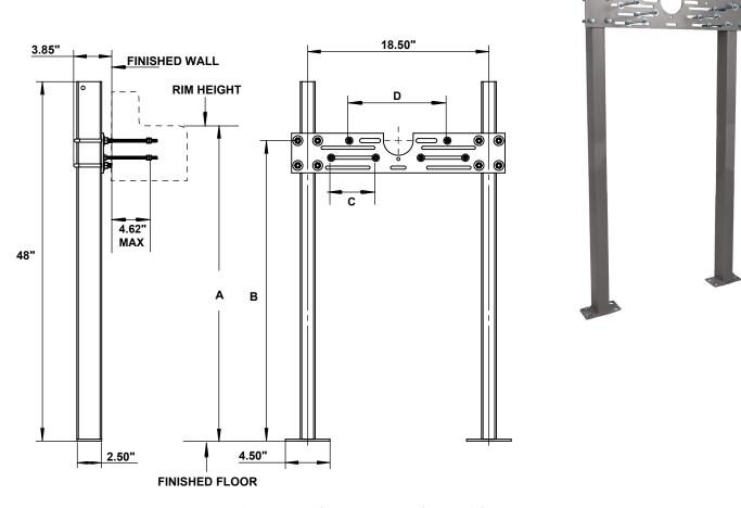
Recommend all feet to be secured to floor with 1/2" bolt and anchors
